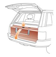
With the upper taildoor open, press the release switch on the top of the lower taildoor, then lower the taildoor.
